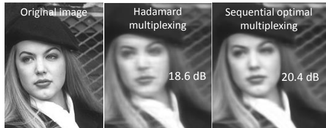
Figure 1. Comparison of Hadamard and Sequential Optimal Multiplexing on Single Pixel Camera based Compressive Imaging ( 16\times compression) shows improved performance for multiplexing matrix that has been designed by taking image and noise statistics into account.
